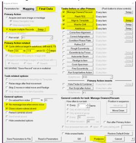
• Align To Template > Setup> new window will open > add label number of BufferP > click ok
