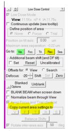
• View - EFTEM, NanoProbe, SA1100x to SA19500 depending on hole size, , Energy Slit in @20ev
