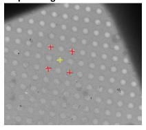
• on Low Dose Control Tile > Define Position of Area > click Focus or Trial > on Position on tilt axis box change to zero
