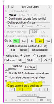
View - EFTEM, Nanoprobe, SA15000× ± one mag, depending on hole size
