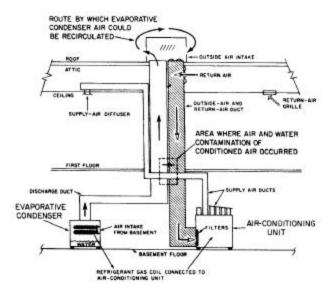
Suspecting that somehow air from the condensing system was contaminating the adjacent air supply duct you set off some smoke bombs in the condensing system ductwork.
